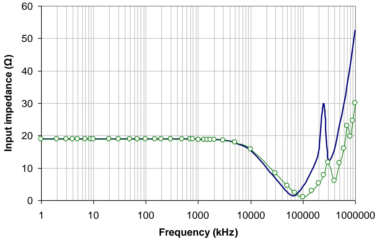
Measured (line with circles) and calculated (solid line) input impedance for 30 mA coaxial shunt at frequencies up to 1 GHz.
