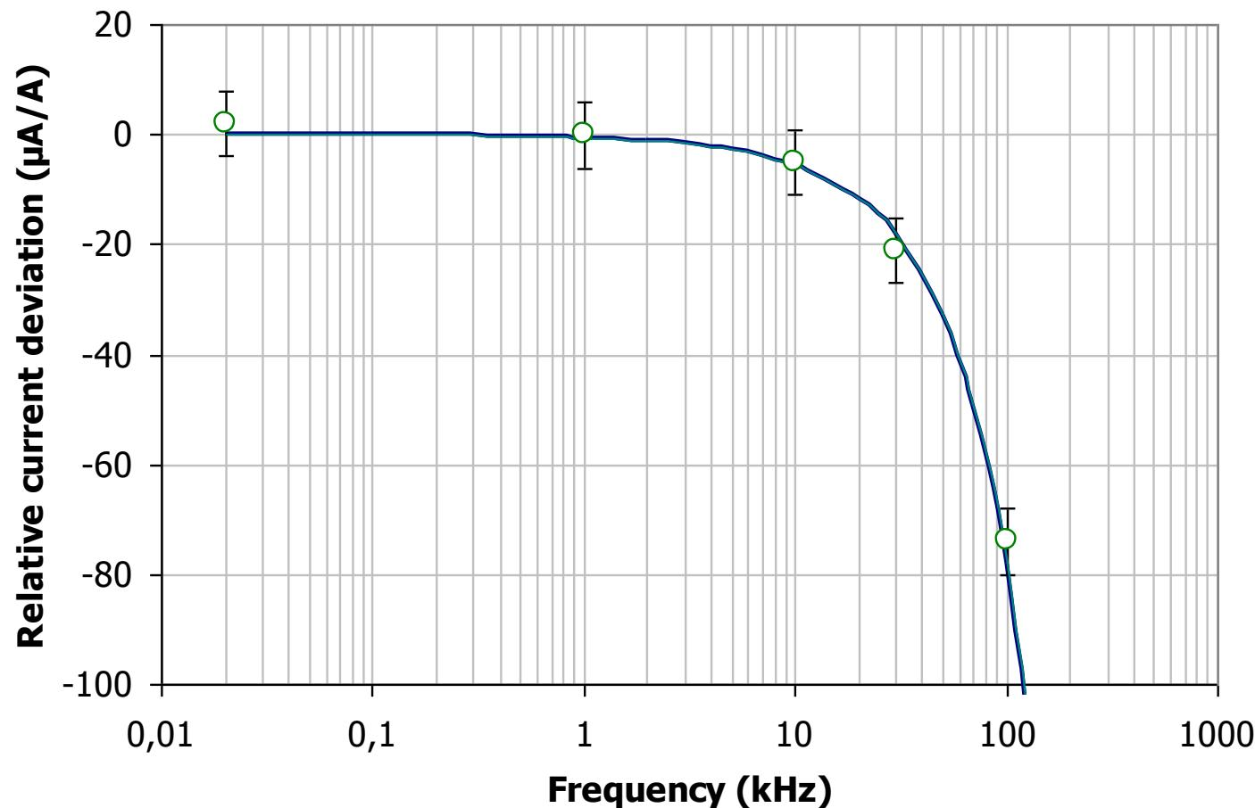
Measured (circles with corresponding  $\pm 6 \mu\text{A}/\text{A}$  uncertainty bars) and calculated (solid line) frequency response of 30 mA current shunt. Measurement were performed up to 100 kHz.
