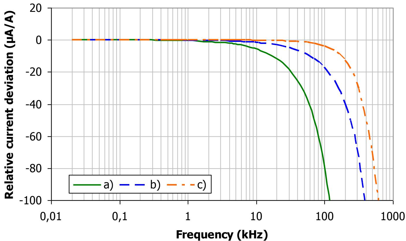
Calculated frequency responses for a) original design, b) design with ten times shorter cross-bars and c) design with both ten times shorter cross-bars and PCB material with ten times lower dissipation factor.
